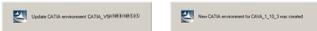
Fig. 2—13: Messages indicating the adaption and the creation of the CATIA environment respectively
